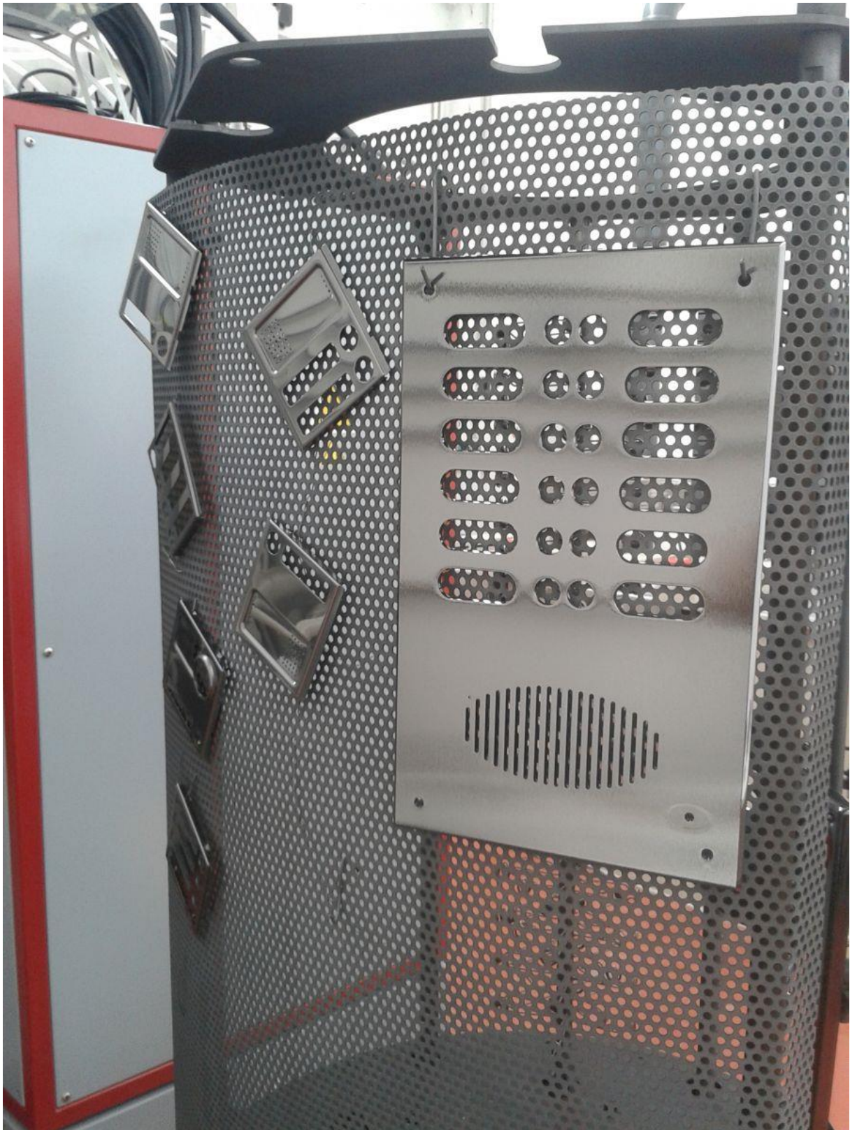
This type of covering is highly resistant to wear and tear and scratching. The essential qualities of a PVD surface treatment are hardness and durability, meeting the specifications of our high end belatec products.
